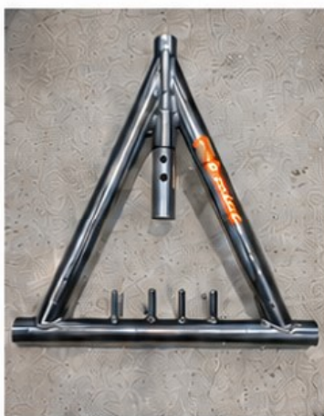
Adjustable height Sill Stands Designed and Manufactured in house at Pro Rally Motorsport.
