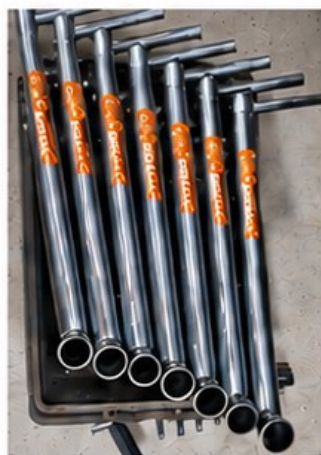
Adjustable height Sill Stands Designed and Manufactured in house at Pro Rally Motorsport.
