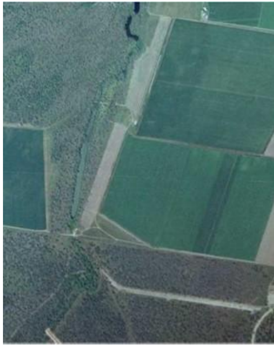
Photo 17. Turbid inflows to the upper catchment lagoon following construction of irrigation scheme tailwater drains (white earthworks in lower part of image) in Apr 1994.
