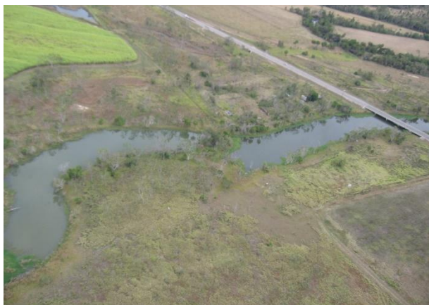
Photo 2. Sustained high water levels within the Didgeridoo Lagoon system. The appearance of features consistent with salt scalds on adjoining frontages, and an apparent decline in the vigour of adjoining floodplain vegetation,
