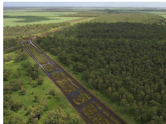
Photo 54. Sunwater drain (RB1) bisecting an area of melon hole/Gilgai floodplain wetland. While these drains lack true riparian vegetation, dedicated management of in-drain vegetation condition – away from aquatic grass weeds and toward emergent native aquatic plants – could deliver potential water quality, habitat, and flow capacity benefits.
