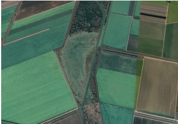
Photo 13. 'Green Swamp' is a state significant natural treeless wetland that historically acted as a detention basin in an area of impeded floodplain drainage and provided bird and other wetland fauna habitat through the wet season. Constructed drains RB1/2A (left) and RB1 (right) now alienate it from inflows in all but flood events.
