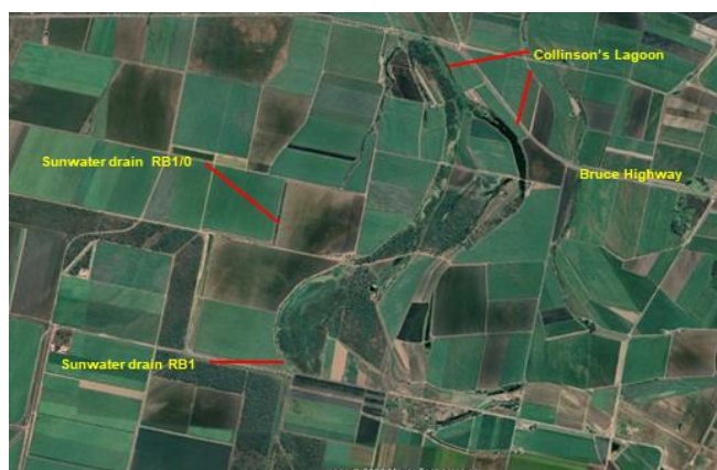
Photo 1. Sunwater tailwater drain (RB1, RB1/0) sources of aseasional inflows to Collinson's Lagoon system. Note water colour upstream (clear black offline from tailwater) versus downstream (turbid brown online to tailwater) lagoons.
