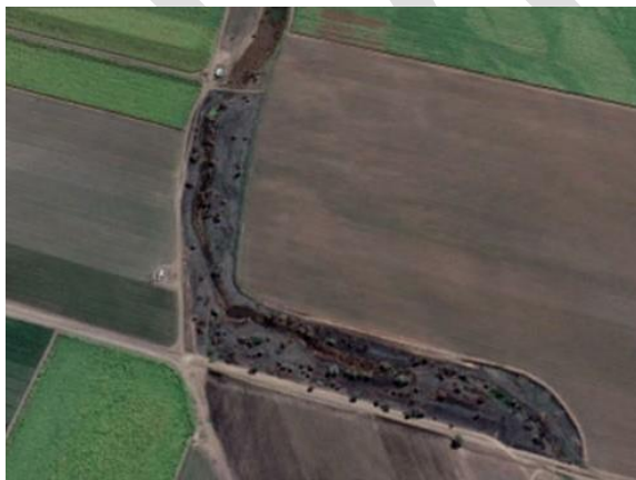
Photo 73. A regularly-burnt distributary reach in the system's eastern catchment that drains north from the Bruce Highway toward Lochinvar. Breaks in cumbungi infestation at this site's northern boundary point to the control capacity of burning, albeit via intense fires.
