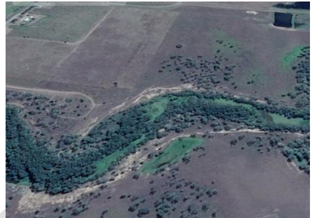
Photo 37. Lower system riparian corridor with cattle pad-generated erosion on dispersive sodic soil levees. The beneficial outcomes of applying cattle grazing pressure as a riparian and wetland habitat management tool need to be balanced with management efforts that limit potential impacts (Tait 2011).
