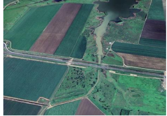
Photo 2. Water flowing to Horseshoe Lagoon (above) from the BHWSS due to irrigation tailwater flows, or catchment rainfall run, is a source of both turbidity and nutrient loading.
