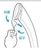
扣紧 Buckle tightly 拆下 Disassemble
