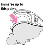
Remove the reel from the water and hold it up with the connector side facing down to ensure that the water completely drains from inside the reel.
