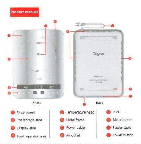
Product model: C-A21MO15 IC-A21M02B IC-A20M015 IC-A20M02B 1C A22M015 IC-A22M028 Rated power: 2100W Rated frequency: 50HZ Rated voltage: 220V Gross weight: 3.5kg Size: 416mm x306mmx45mm
