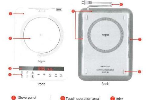
Product model: 0-A2102 / 2103/2104/2107/2108 / A21SWFO5 TG-S2101 / 2102 Rated power: 2100W Rated frequency 50HZ Rated voltage 220V-Gross weight: 3.3kg Size: 410mmx300mm x 39mm
