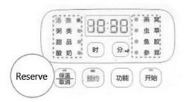
Press the "reservation" key, the time display area is the default reservation time of the function (that is, the default cooking time), and then press the "hour and minute" key to adjust the required time.
