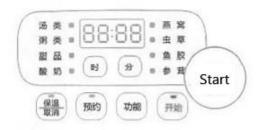
Press the "Start" button, the indicator light changes from flashing to a long stew pot to start cooking
