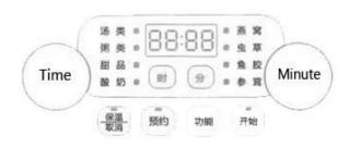
Each function menu has a default cooking time, but it can also be adjusted by pressing the "hour" and "minute" keys as needed.
