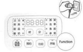
Close the upper cover, plug in the power source, press the "function" button to select any function menu and heat it for about 5 minutes.
