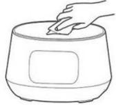
Wipe the inner surface of the water tank with a damp cotton cloth and repeatedly rinse the water tank with clean water to remove the vinegar smell.
