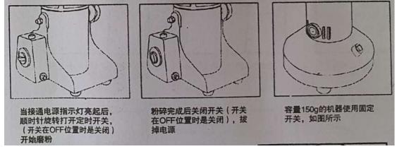
When the power-on indicator lights up, turn on the timing switch clockwise (when the switch is OFF, it is off) to start grinding.
