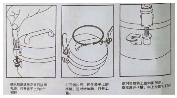
After confirming that the machine is powered on normally, unplug the power supply and open the two locks on the cover
