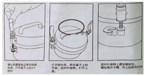
After confirming that the machine is powered on normally, unplug the power supply and open the two locks on the cover
