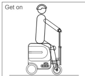
Sit on the case, adjust the center of gravity, place both feet on the pedal
