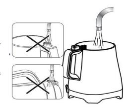
■切忌将桶底浸入水中;请勿用水冲洗耦合器、电源插口,以防进水,发生危险。 Do not immerse the bottom of the bucket in the water; do not wash the couplers with water, power Jack, to prevent water intake, dangerous.
