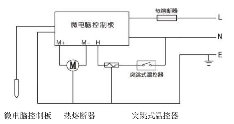
Microcomputer control board, Thermal cut-off, Sudden hop thermostats
