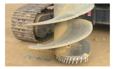
The auger that is used to drill the shaft
