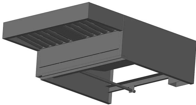
The vapour condensation system consists of a finned labyrinth that allows for the development of a very large exchange surface, positioned in such a way as to appropriately force the air flow path, with the purpose of condensing the vapours coming from the cooking chamber and from oven outlet when the door is opened.
