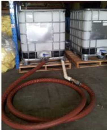
Insert the Plastic pipe end of the hose to the black bin(s). Turn on the flow by twisting the valve.
