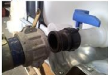
Attached female end of hose couple to tank
