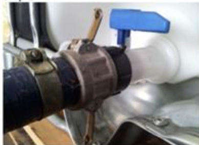
Ensure the coupling is firmly attached into the tank outlet.
