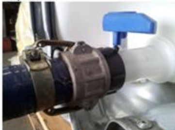
Once attached, pull lever on sides backwards to lock the hose in lock position
