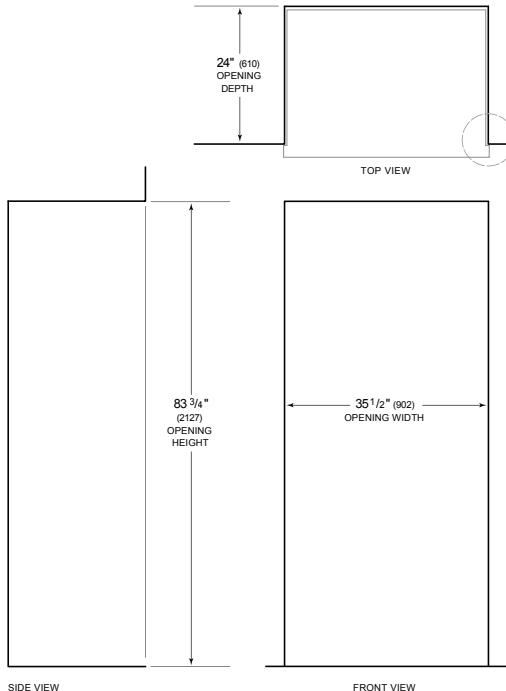
NOTE: 3 1/2" (89) finished returns will be visible and should be finished to match cabinetry
