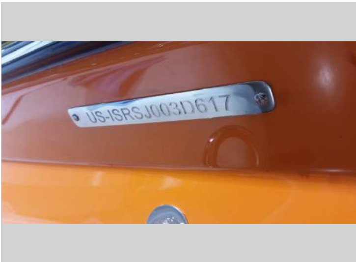
The hull identification number is located on the upper right hand side of the transom below the rub rail.
