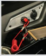
Your Supra is equipped with a Safety Lanyard/Engine Shut Off switch. In order for the engine to run, the plastic tip of the safety lanyard must be attached to the switch. If the clip is removed from the switch, the engine will not run.
