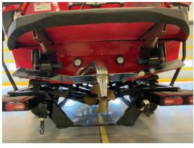
The distance between the boat and the wheel runner board should be equal on both sides.
