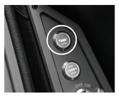
The Horn Switch is located on the starboard switch panel. Sound the horn by depressing the button.
