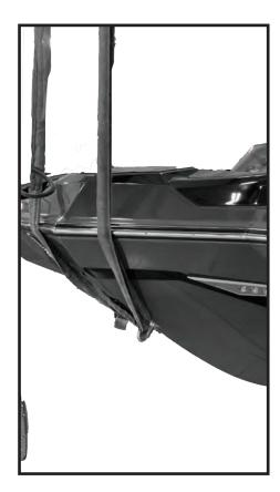
NOTE: For boat houses, we highly recommend the use of a lifting cradle. Cradle bunk design should mimic the bunk design of the trailer.
