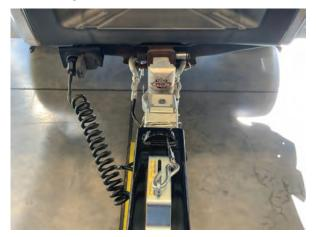
NOTICE: If your hitch ball has an excessive flat spot on top, the latch may not engage properly. If the latch does not catch, check with your dealer or hitch installer before trailering.
