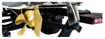
The SmartPlate allows the driver to control the running attitude of the boat. It is integrated and logically controlled by the Supra Vision Control System to automatically deploy and retract to preset positions based on boat speed and other parameters. It can also be controlled manually by buttons on the back side of the steering wheel or the center touch screen above the steering wheel.
