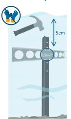
Hammer your waratah into the stream bed, in an area of moderate to high flow.
