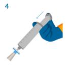
Insert the plunger and push as much slurry as possible through the filter until the filter is clogged, discarding the outlet slurry. Don't worry if you can only get a small amount of liquid through the filter.
