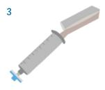
Remove the plunger from the large syringe, screw on the blue filter, and pour the slurry into the empty syringe barrel.
