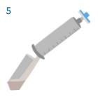
Remove the plunger and pour any remaining slurry back into the falcon tube, which can then be capped. The falcon tube can then be disposed of or frozen for future analysis.
