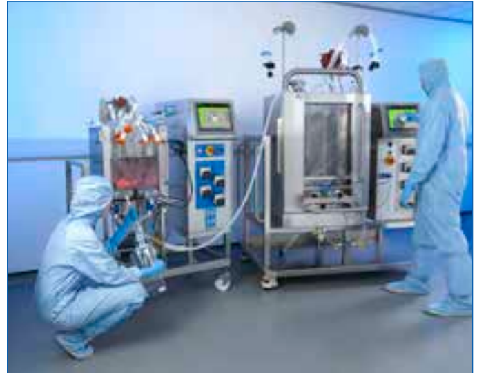
Setting up a transfer from an Allegro STR 50 L bioreactor to an Allegro STR 200 L bioreactor
