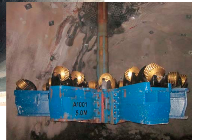
▶ A reamer head is attached to the drill string to bore out the shaft from the bottom upwards.
