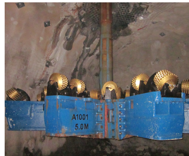
Above: The large cutting head of a raise borer which will be used to ream out the new 5.5m wide ventilation shaft.
