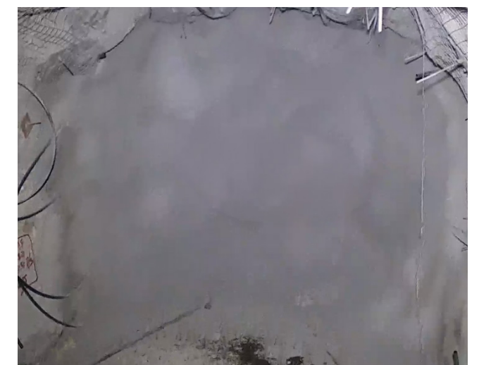
Step 3: Once the paste has been placed, we call it a Paste Wall or "Bulkhead".
